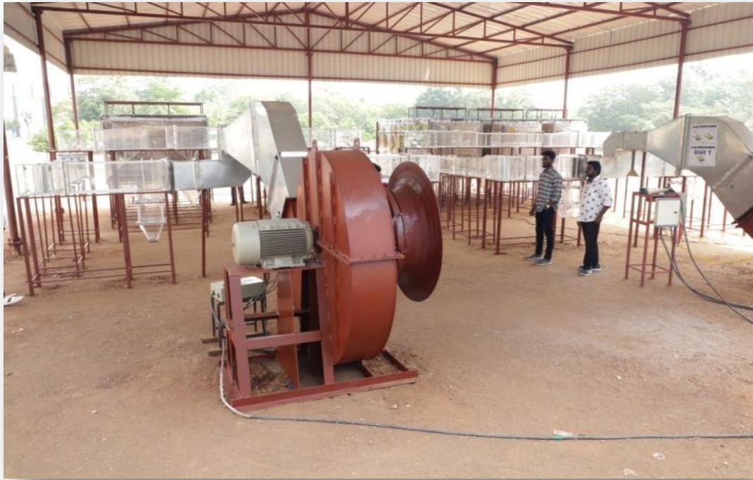
Figure 2 1:10 Scale Physical Model of Electrostatic Precipitator of 3x210MW Mejia Power Plant
