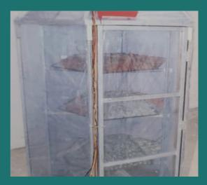
A key feature of the EHPP solar dryer is its capability to evenly distribute hot air throughout the drying chambers, ensuring consistent drying across all produce and minimizing the risk of uneven drying and spoilage. Moreover, with the inclusion of an electronic controller setup and six thermostats, precise temperature control is achieved, optimizing drying conditions for enhanced efficiency and quality.
